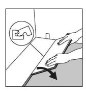
Place the first plank of the new row with the tongue side at an angle against the groove side of the plank in the previous row. Press forward and lay it flat at the same time.
