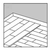
Turn the tongue side of the plank facing the wall. Maintain a gap of 5mm (0.2") on the short side.
