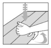
Do not bend connected planks backwards as this will damage it.
