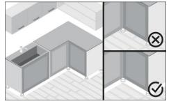
Any permanent and heavy structures like kitchen islands or cabinets should be installed first and not on top of Floating floors, as they should be able to move around such heavy objects, otherwise it could lead to open joints or separating or damaged planks.
