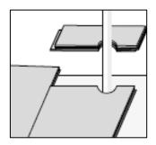
Cut the plank with a 45° angle towards the hole. The cut--off piece is glued in the position again.
