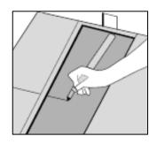
Cut the final plank of the first row to the correct length. Place the final plank face down and the short side without the locking strip towards the wall. The distance to the wall should be 5mm (0.2")
