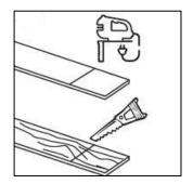
Make sure that the long sides of the planks make a straight line. Use the cut piece of the plank from the previous row to start the next one.
