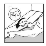
Lift the plank (together with the previous one laid in the same row) slightly up (about 30mm (1.2"), push it against the row in front and then put it down.
