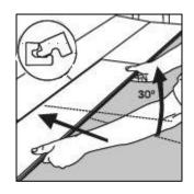
Adjust the distance to the wall to 5mm (0.2") when three rows are complete.
