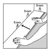
Hold the next plank against the first at an angle to the first one and lay it flat on the floor.
