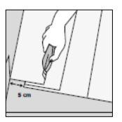
The last and first plank can be cut in the correct width.
