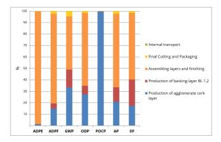
According to the graph above, the processes of the products Cork Flooring Floating with high resistance varnish (WRT) and with UV varnish (WPS) with the highest impacts are the production of the agglomerate cork layer and assembling and finishing.
