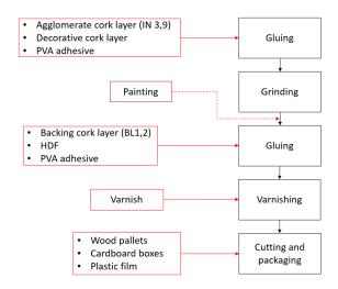
The manufacturing process of the flooring product begins by assembling the agglomerate cork layer and the decorative layer using a cold-melt adhesive. Then the decorative cork layer is painted and these components are blended with the layers of HDF and BL 1,2, using the cold-melt adhesive. The final layer is the varnish and the resulting board is then cut into the defined dimensions and is now ready for packaging and storage.
